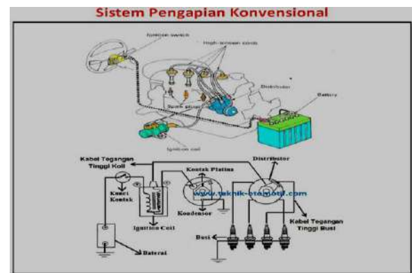
Gambar 2. Diagram Sistem Pengapian Konvensional
